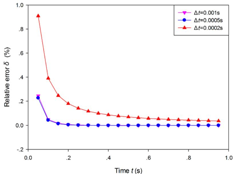
**Figure 3:** The relationship between time step  $\Delta t$  and relative error  $\delta$
