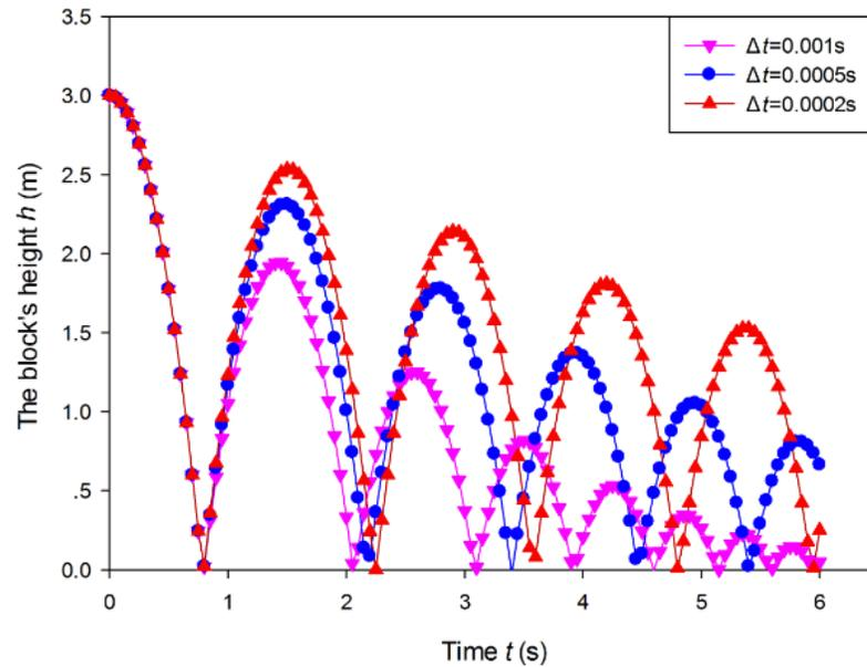
**Figure 9:** The relationship between the block's height  $h$  and time step  $\Delta t$
