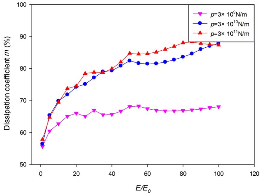
**Figure 10:** Dissipation coefficient  $m$  with different  $E$  and  $p$
