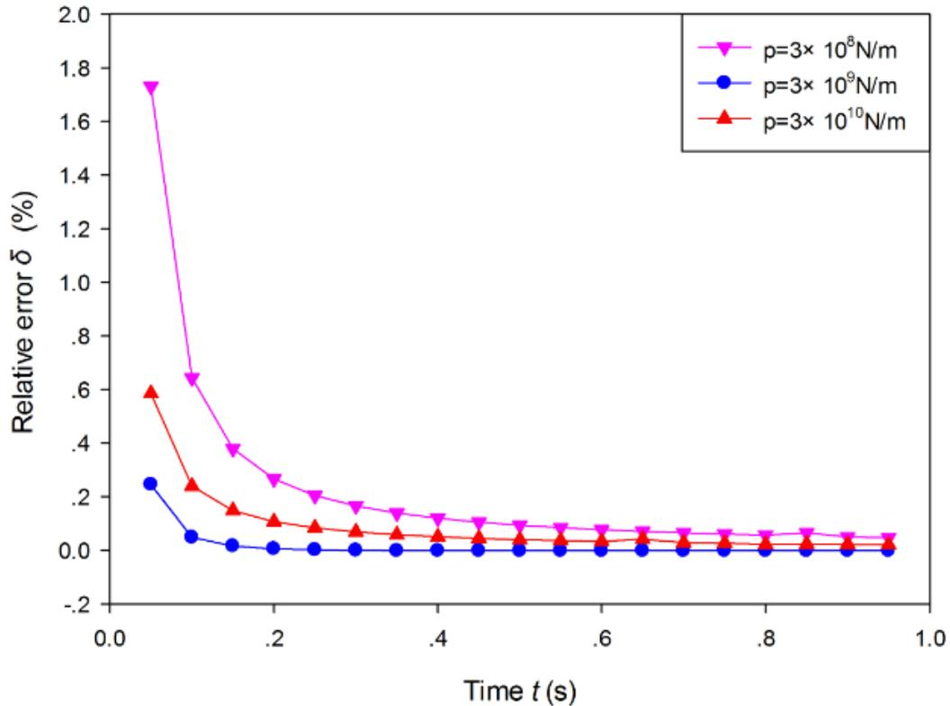
**Figure 4:** The relationship between spring stiffness  $p$  and relative error  $\delta$
