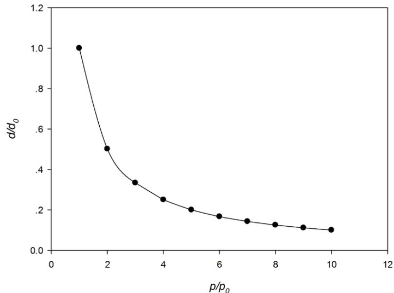
**Figure 7:** The relationship between spring stiffness  $p$  and balanced position  $d$
