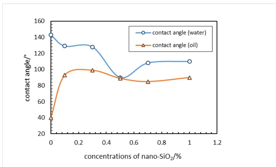
**Figure 3:** The water-oil phase contact angle of rocks soaked by nanometer SiO<sub>2</sub> with different concentrations and FP415 of 1% concentration.
