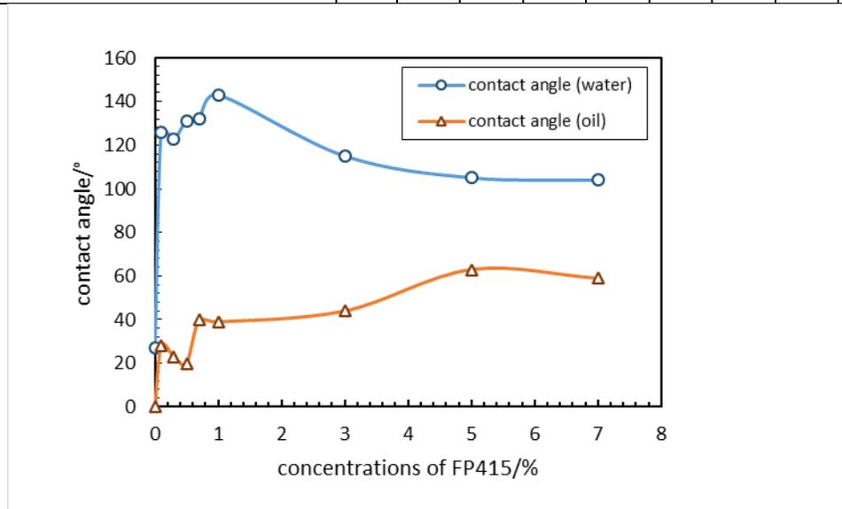
**Figure 2:** The gas phase contact angle of rocks soaked by FP415 with different concentration
