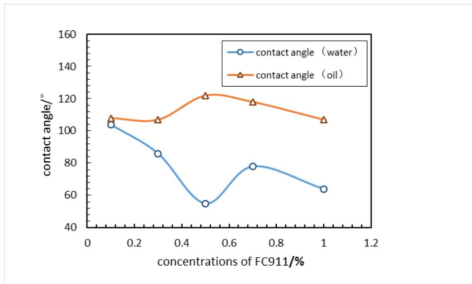
**Figure 4:** The contact angle of rocks soaked by different concentrations of FC911 and FP415 of 1% concentration and nanometer SiO<sub>2</sub> of 0.3% concentration.
