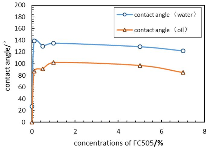
**Figure 5:** The contact angle of rocks soaked by different concentrations of FP505.
