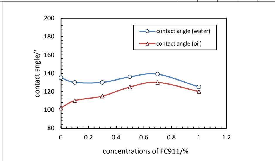
**Figure 7:** The contact angle of rocks soaked by different concentrations of FC911 and FP505 of 1% concentration.
