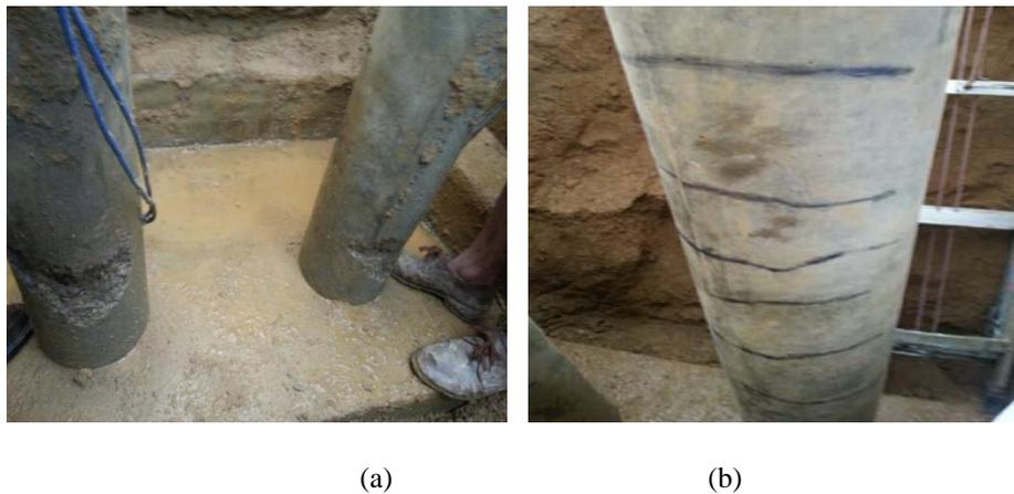
**Figure 5:** The test processes: (a) before loading; (b) fractures on pile body.
