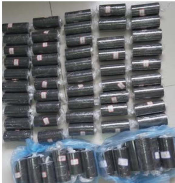
**Figure 1:** Coal specimens
