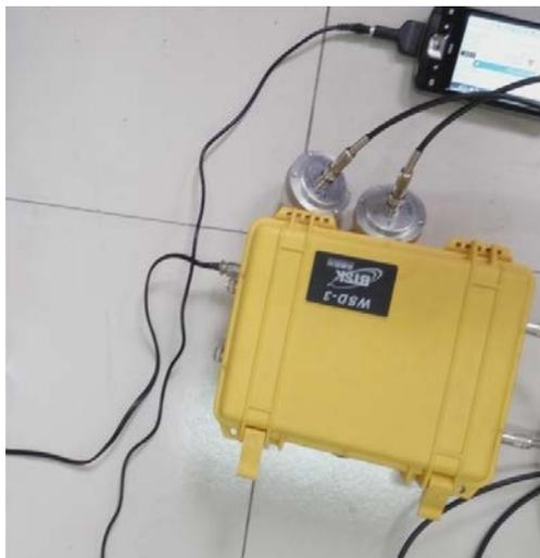
**Figure 2:** Wave velocity measuring instrument
