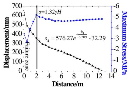
**Figure 13:** Evolution curves of stress and displacement in left bottom corner strata
