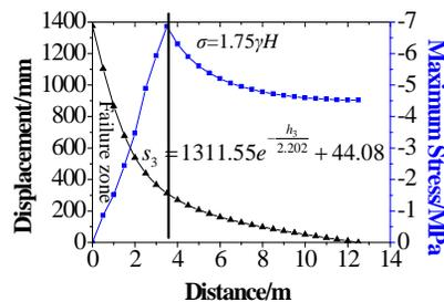
**Figure 10:** Evolution curves of stress and displacement in right base arch strata
