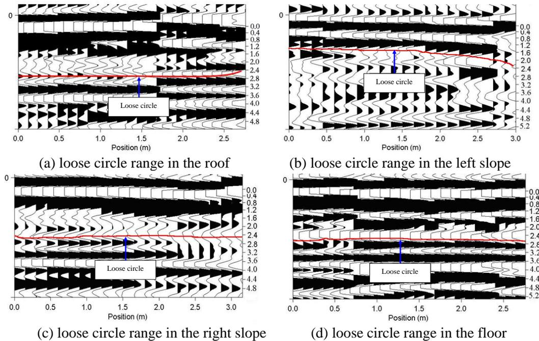
**Figure 15:** Measurement results of roadway surrounding rock by radars
