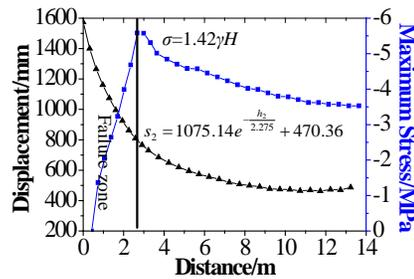
**Figure 8:** Evolution curves of stress and displacement in right shoulder strata
