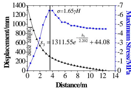
**Figure 11:** Evolution curves of stress and displacement in left base arch strata
