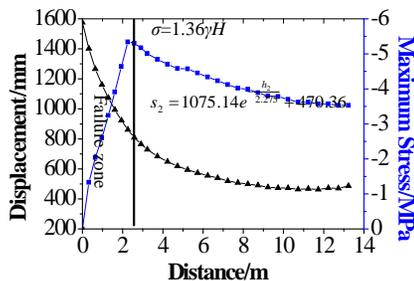
**Figure 9:** Evolution curves of stress and displacement in left shoulder strata
