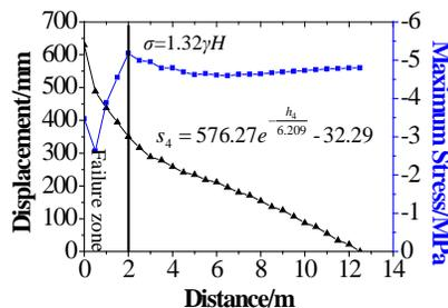
**Figure 12:** Evolution curves of stress and displacement in right bottom corner strata
