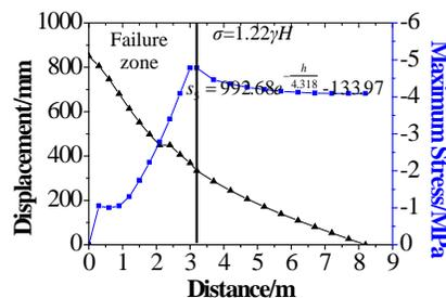
**Figure 14:** Evolution curves of stress and displacement in floor strata
