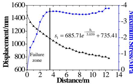
**Figure 7:** Evolution curves of stress and displacement in roof strata
