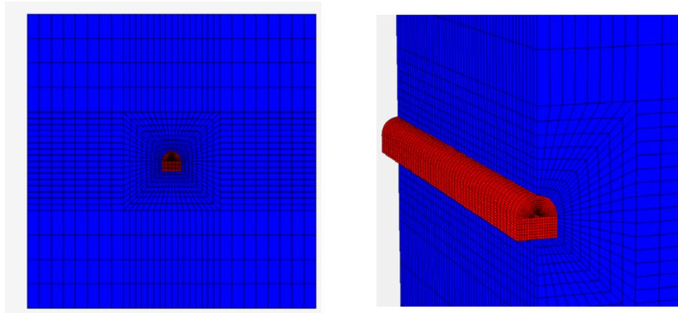
**Figure 3:** Numerical calculation model of the rock roadway
