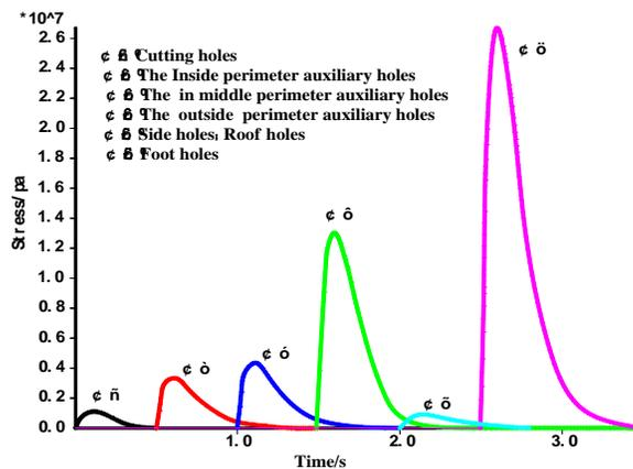
**Figure 6:** Approximately equivalent dynamic load versus time applied to surrounding rock of the driving face floor
