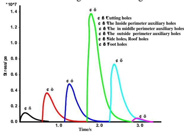
**Figure 5:** Approximately equivalent dynamic load versus time applied to surrounding rock of tunnel roof and wall
