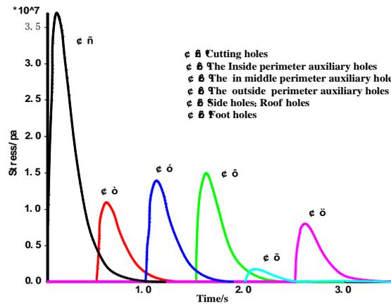
**Figure 4:** Approximately equivalent dynamic load versus time applied to surrounding rock of heading face
