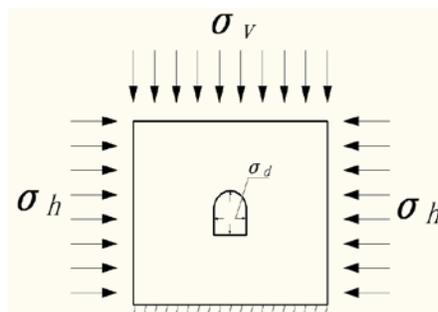
**Figure 1:** Mechanical model of the deep rock roadway
