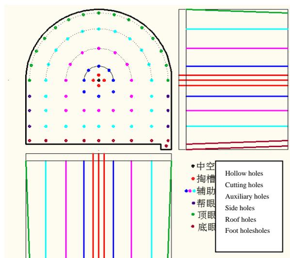
**Figure.2:** Layout of the blast holes in the driving face
