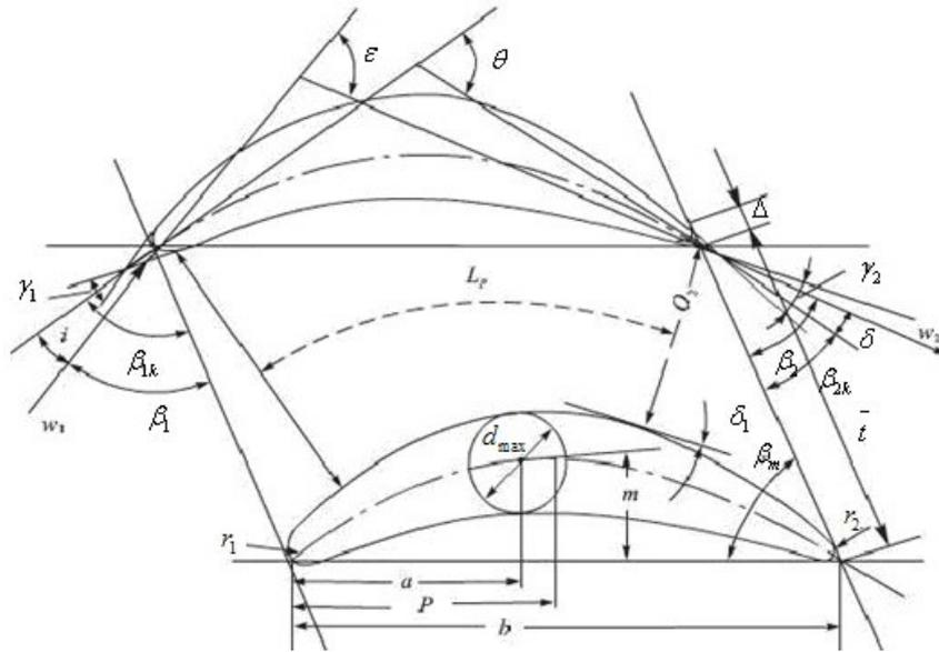
**Figure 1:** Geometric parameters of a single blade [8]
