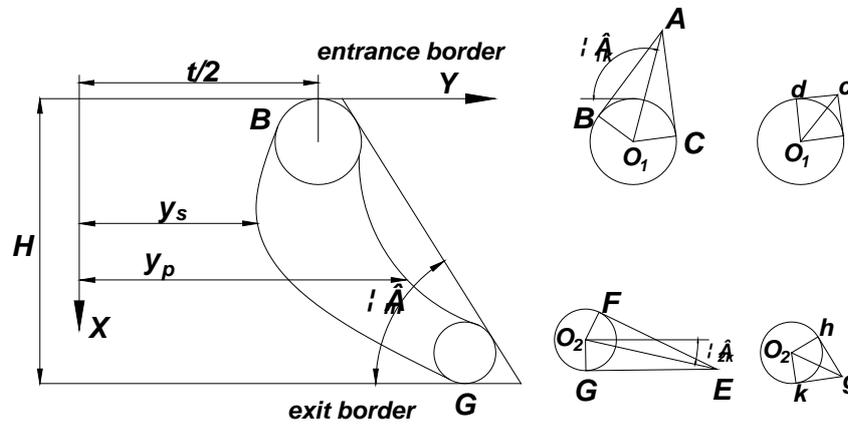
**Figure 2:** Rectangular coordinate system of blade profile [8]
