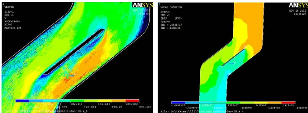
**Figure 5:** velocity lines and pressure contour of straight blade
