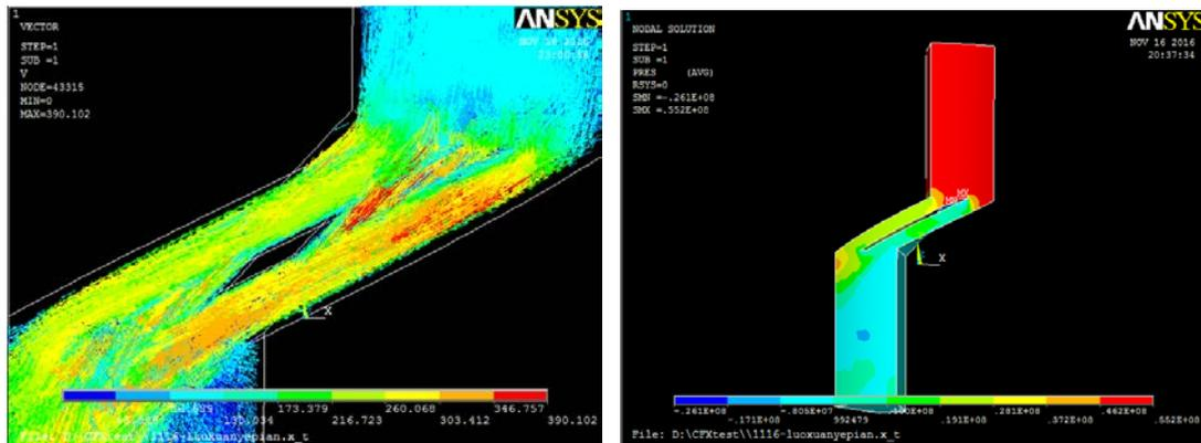
**Figure 6:** Velocity lines and pressure contour of helical blade
