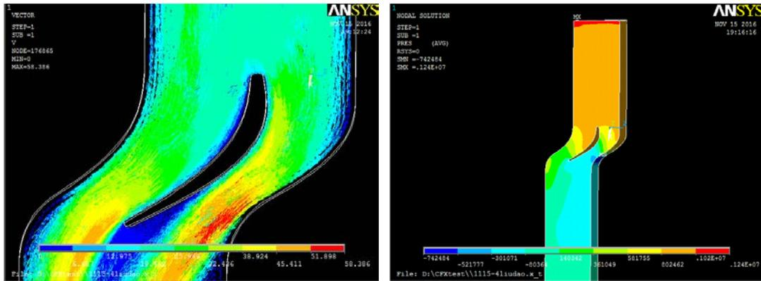
**Figure 4:** velocity lines and pressure contour of quantic polynomial blade
