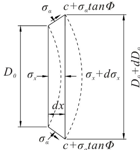
**Figure 5:** Small element of plastically deforming ground (EBB'E')
