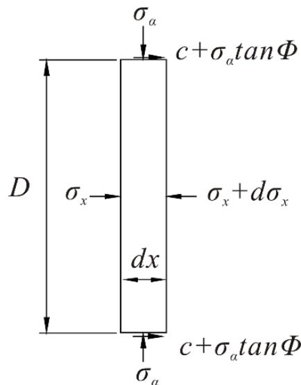
**Figure 4:** Small element of plastically deforming ground (AEE'A')
