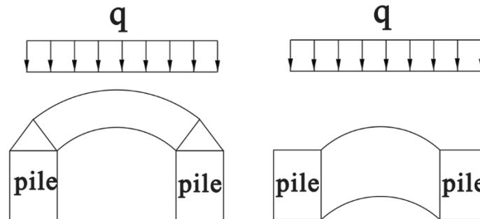
**Figure 1:** Sketch of the soil arching between piles
