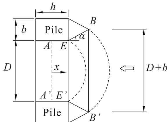
**Figure 3:** State of soil arching in the ground just around piles
