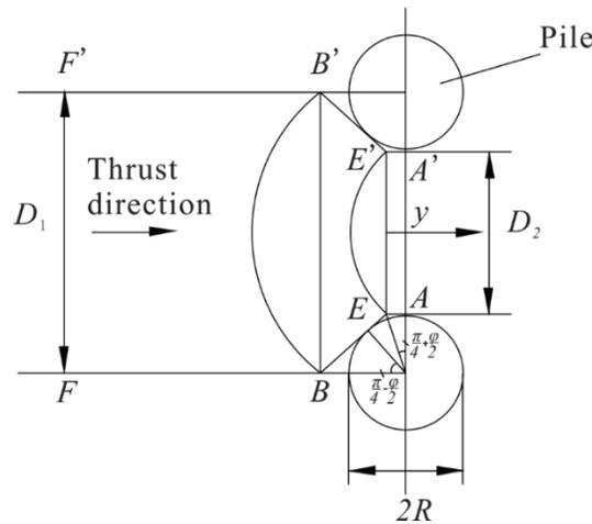
**Figure 2:** State of plastic deformation in the ground just around piles
