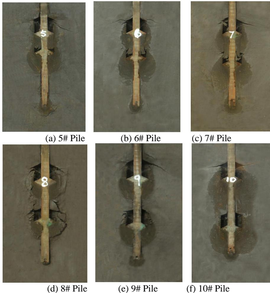
**Figure 5:** The ultimate failure state of soil around the pile with different plate space
