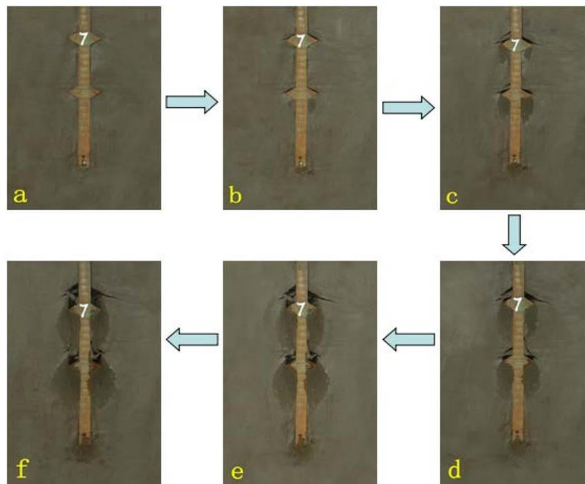
**Figure 4:** The failure process of soil around the pile of 7# pile
