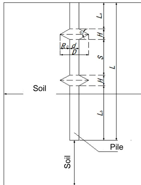
**Figure 1:** The sketch map of pile and soil
