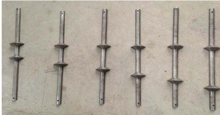
**Figure 2:** The half-section test pile with different plate space
