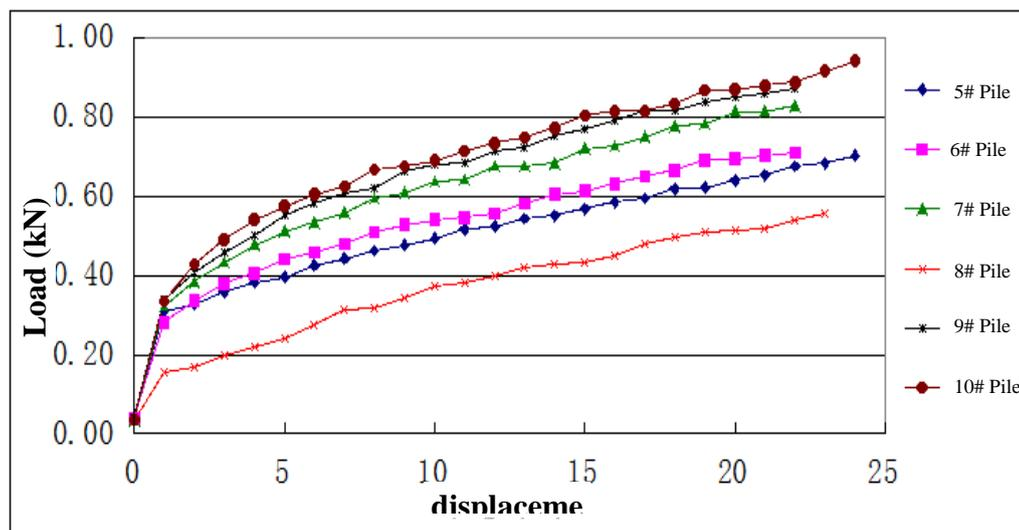
**Figure 6:** The displacement-load curve comparison chart of testing pile with different plate space
