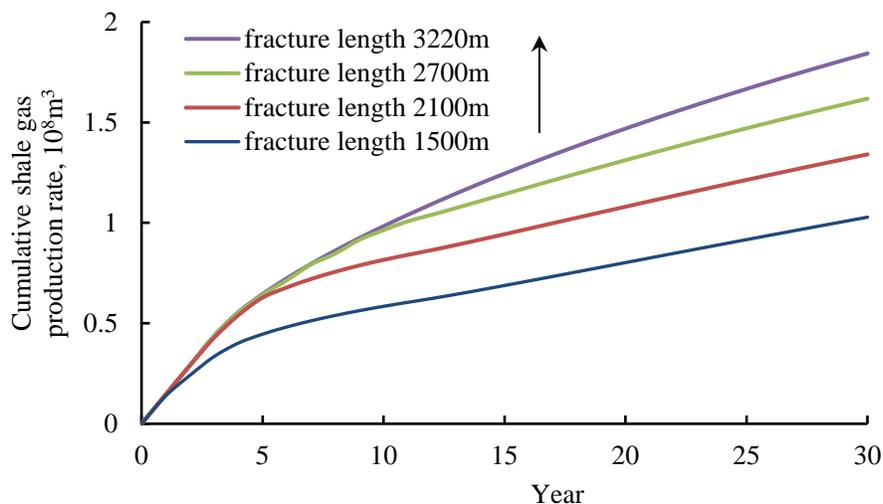
**Figure 9:** Influences of fracture total length on cumulative shale gas production rate
