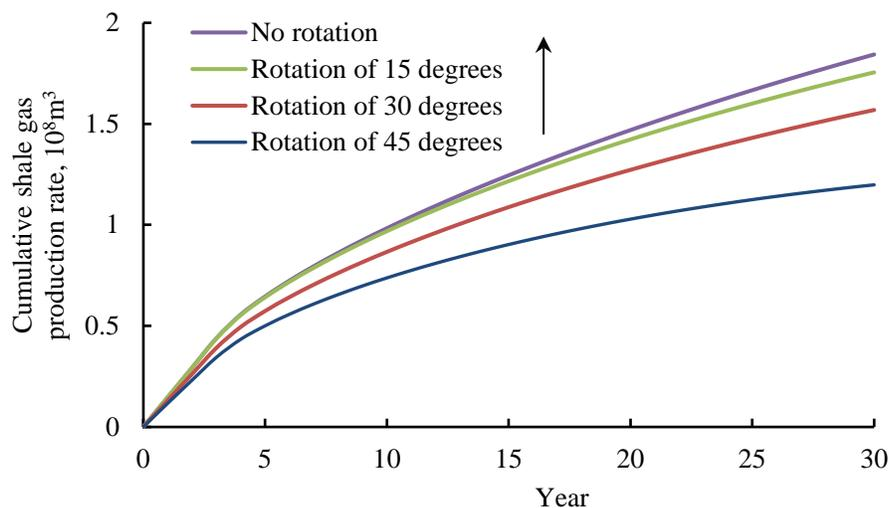
**Figure 10:** Influences of fracture orientation on cumulative shale gas production rate
