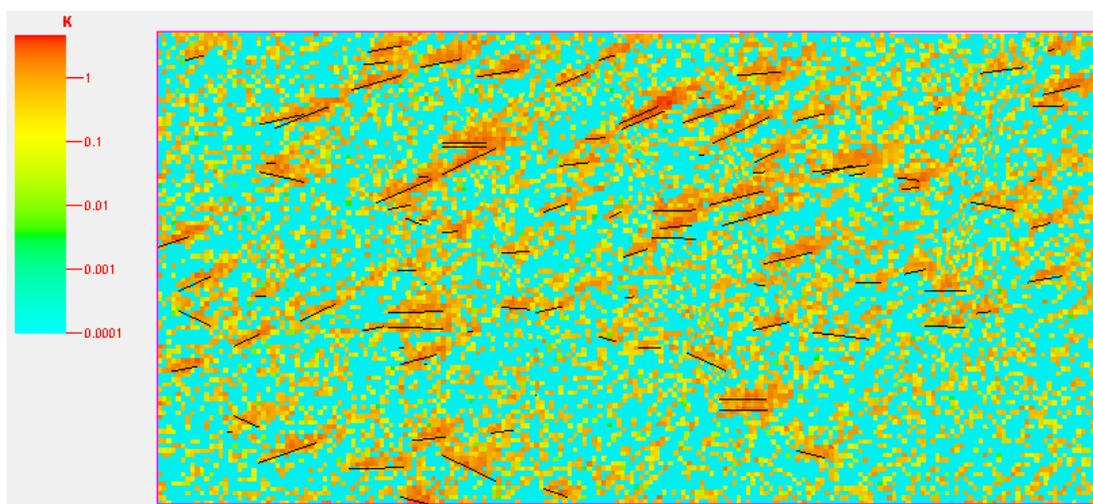
**Figure 4:** Correlation between natural fracture distribution and permeability distribution
