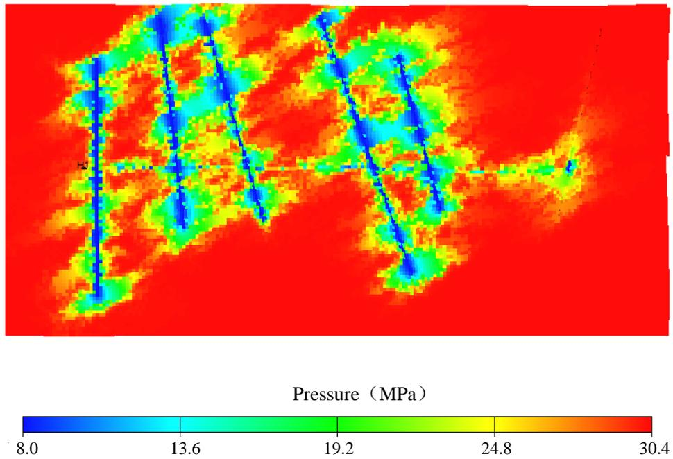
**Figure 7:** Pressure distribution of fractured horizontal well in shale gas reservoir (5 years later)
