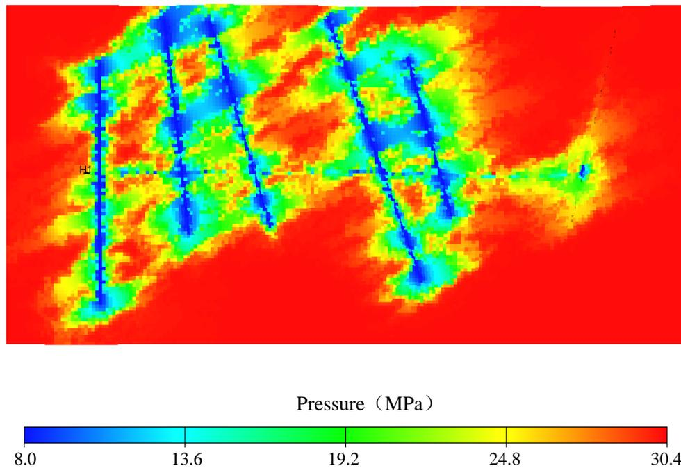
**Figure 8:** Pressure distribution of fractured horizontal well in shale gas reservoir (10 years later)
