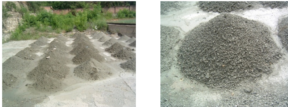
Figure 10: Consolidated tailings pile after dewatering
