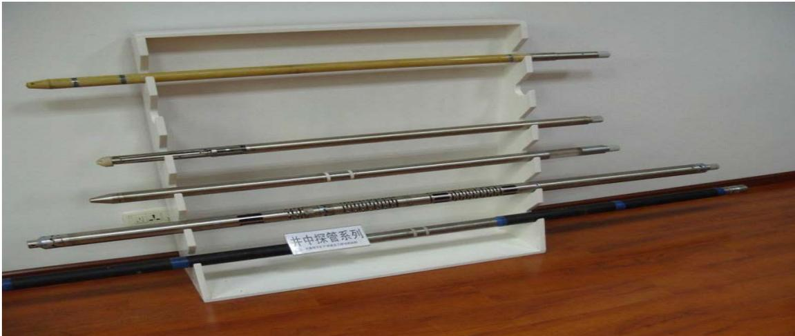
**Figure 2:** Logging probes with various dimensions used in mineral and oil exploration
