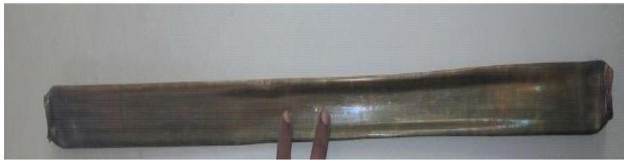
**Figure 5b:** Collapse of brass tube of 0.6 mm thickness buckled at 25 kg/sq.cm.
