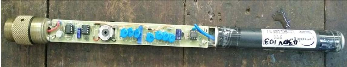
**Figure 1:** Logging probe hosting Geiger Muller counter and associated electronics used for gamma ray spectra in a borehole
