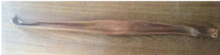
**Figure 5a:** Collapse of copper tube of 0.6 mm thickness buckled at 20 kg/sq.cm.
