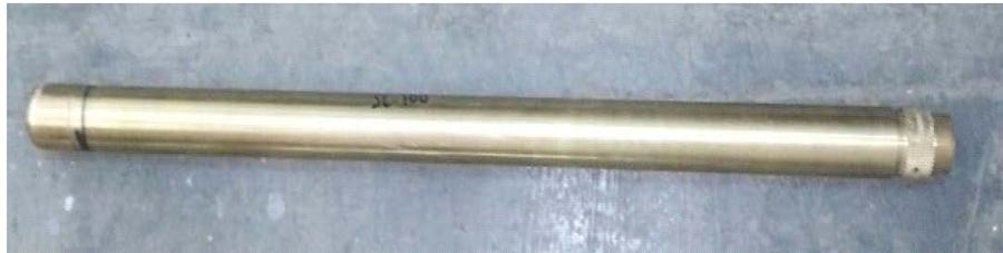
**Figure 5c:** Non Collapse of brass tube of 1.6 mm thickness that buckles at ~ 98 kg/sq.cm.
