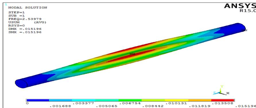
**Figure 3a:** Copper pipe of thickness of 0.6 mm, the collapse pressure is observed to be  $25.397 \text{ kg/cm}^2$
