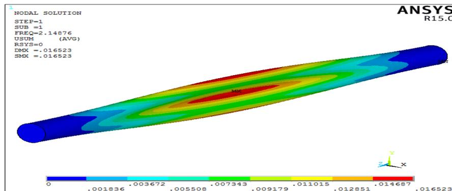
**Figure 3b:** Brass pipe of thickness 0.6 mm, collapse pressure is observed to be  $21.4876 \text{ kg/cm}^2$
