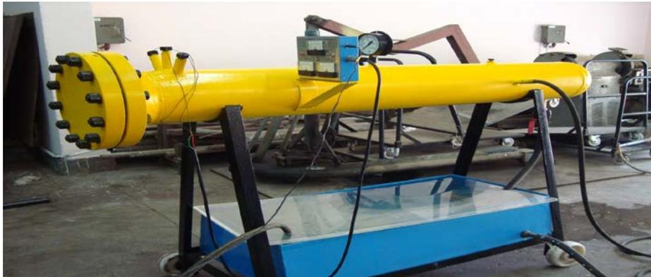
**Figure 4:** Pressure vessel that can withstand an internal pressure of 70 kg/sq.cm.( vessel can with stand a pressure of 97 kg/cm<sup>2</sup>, but it is limited by the flanges that can withstand only 70 kg/cm<sup>2</sup>.)
