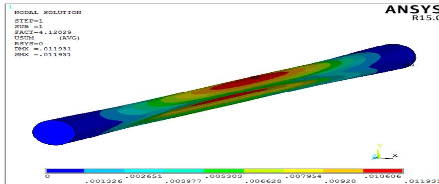
**Figure 3 c:** Stainless Steel pipe of thickness 0.6 mm Collapses pressure is 41.203 kg/cm<sup>2</sup>
