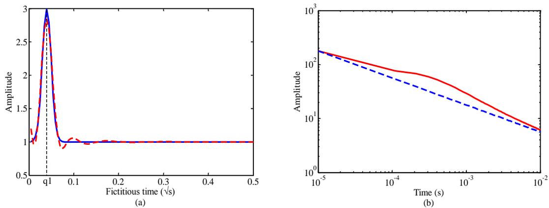
**Figure 1:** This is Results of the fictitious wave field transformation and inverse transformation of the D-type model (a) Synthetic fictitious wave field record of the D-type model and its results of the inverse transformation. The amplitude of pulse is  $A_1=2$ , the width is  $w_1=0.05$ , and the pulse peak fictitious time is  $q_1=0.04$ . (b) Decay curve of TEM signal of the D-type model.
