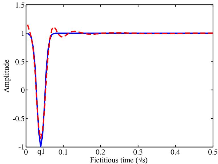
**Figure 2:** Synthetic fictitious wave field record of the G-type model and its results of inverse transformation. The amplitude of pulse is  $A1=-2$ , the width is  $w1=0.05$ , and pulse peak fictitious time is  $q1=0.04$ .
