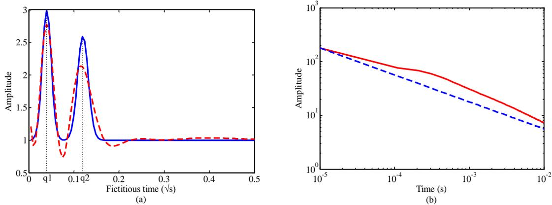
**Figure 3:** Results of the fictitious wave field transformation and inverse transformation of the Q-type model (a) Synthetic fictitious wave field record of the Q-type model and its results of inverse transformation. The first pulse amplitude is  $A1=2$ , the width is  $w1=0.05$ , and pulse peak fictitious time is  $q1=0.04$ . The amplitude of second pulse is  $A2=1.6$ , the width is  $w2=0.06$ , and pulse peak fictitious time is  $q2=0.12$ . (b) Decay curve of TEM signal of the Q-type model.
