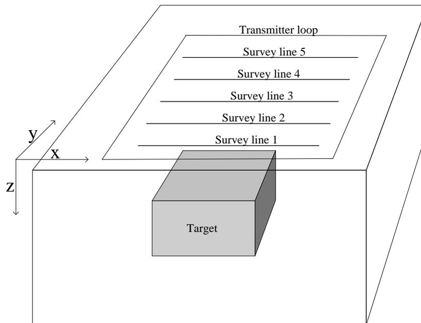
**Figure 4:** Low resistivity target into a half space and the surface line. The gray block in the figure is the underground target, the size is  $80 \text{ m} \times 80 \text{ m} \times 50 \text{ m}$  and the buried depth is  $100 \text{ m}$ . The line space and point distance are both  $20 \text{ m}$ .
