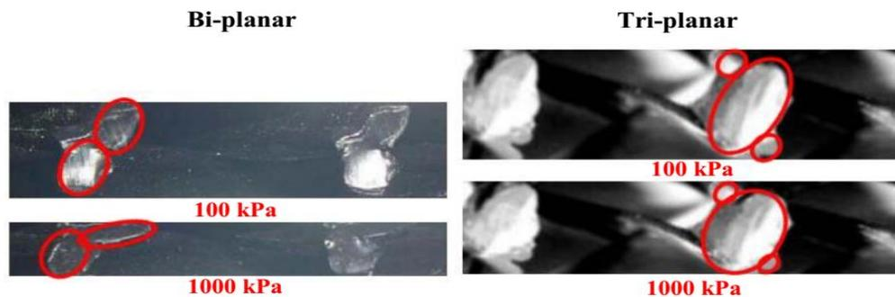
**Figure 6:** Bi-planar and tri-planar geonet samples under compressive stress of 100 and 1000kPa
