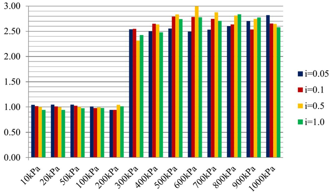
**Figure 4:** The ratio of drainage capacity of the tri-planar geonet sample to that of the bi-planar sample for different values of compressive stress and hydraulic gradient
