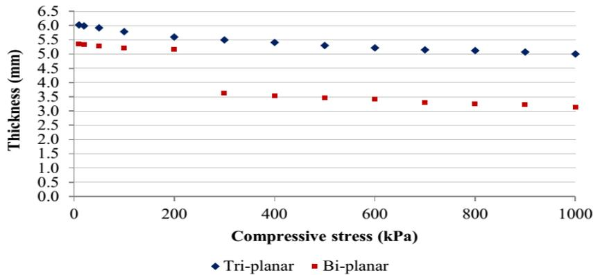
**Figure 5:** Thickness of tri-planar and bi-planar geonet samples versus compressive stress
