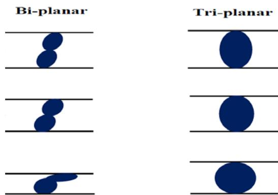
**Figure 7:** Schematic view of ribs deformation pattern for bi-planar and tri-planar geonets
