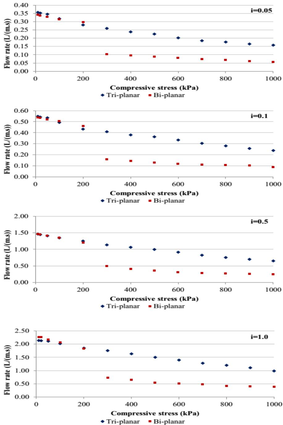
**Figure 3:** In-plane flow rate of tri-planar and bi-planar geonet versus compressive stress
