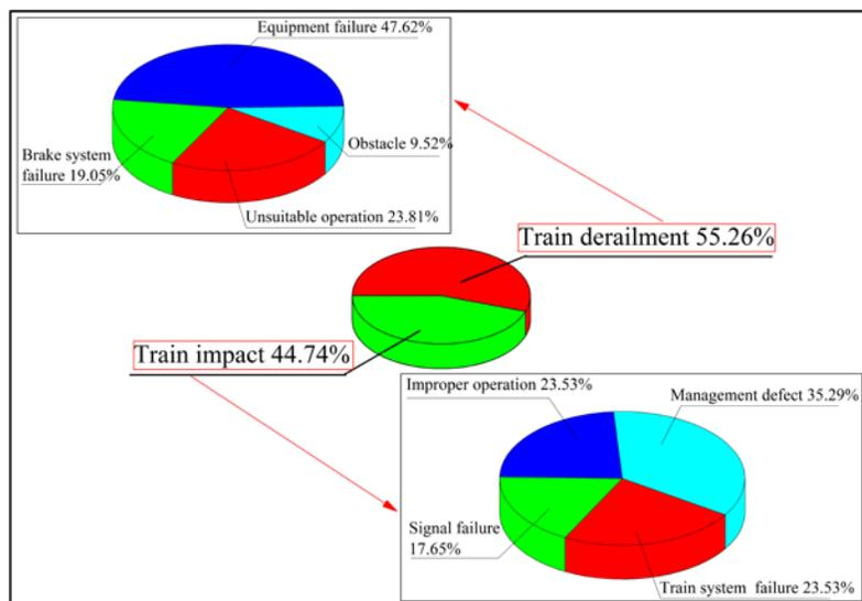
**Figure 8:** Cause distribution of train derailment and impact
