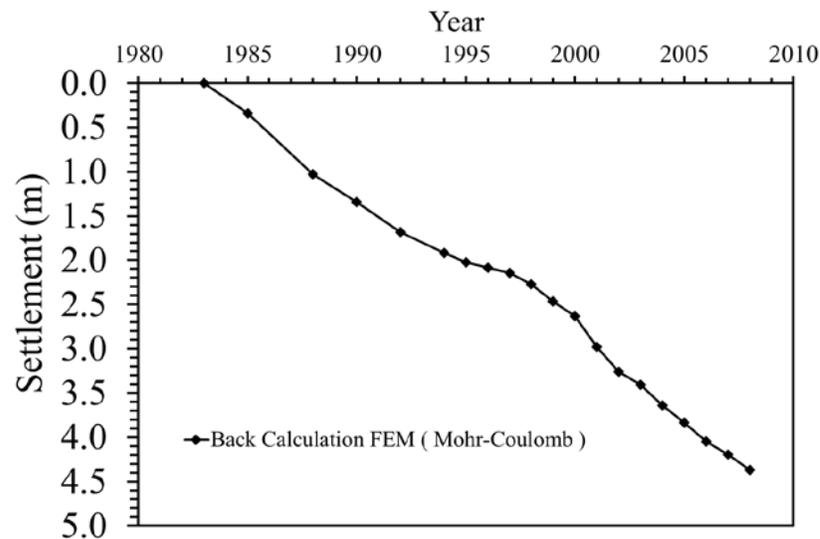
**Figure 3:** Estimating subsidence using the corrected model for a 25 years period of 1983 to 2008
