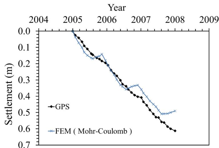
**Figure 2:** Correcting Mohr-Coulomb model using recursive analysis
