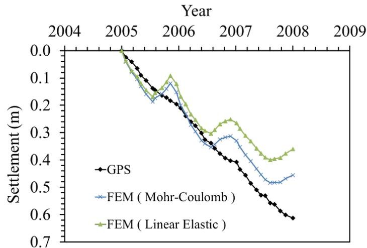
**Figure 6:** Comparing the subsidence value obtained from the primary model and the observations (GPS) between 2005 and 2007.
