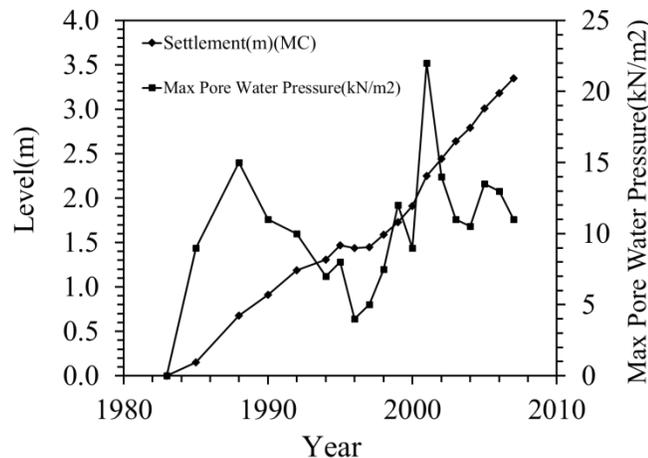
**Figure 4:** Soil surface subsidence and maximum pore water pressure in soil media according to the analysis of Kalate Barfi piezometer's (H) annual data, using primary Mohr-Coulomb model.
