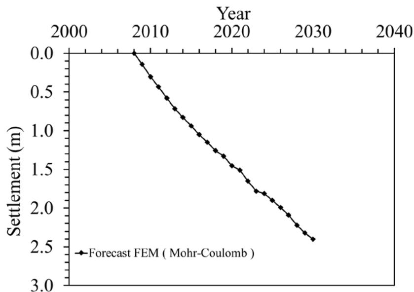
**Figure 4:** Predicting subsidence for the next ten years (2008 to 2030) assuming annual groundwater level drop of 1.5 meters using the corrected model.
