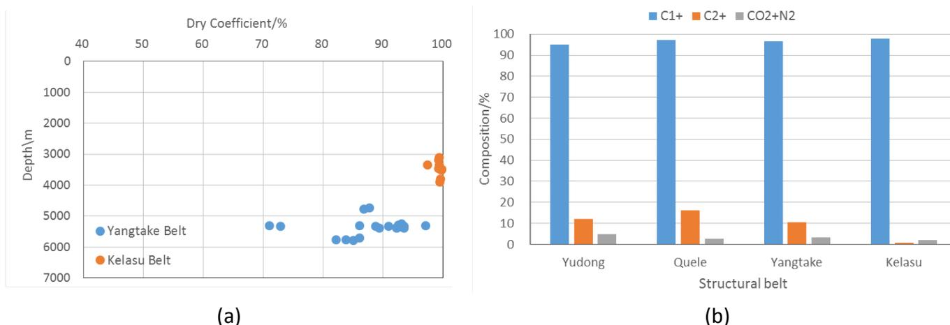
**Figure 2:** (a) Dry coefficient with depth of Yangtake and Kelasu belts, (b) comparison of natural gas composition of different structure belts.
