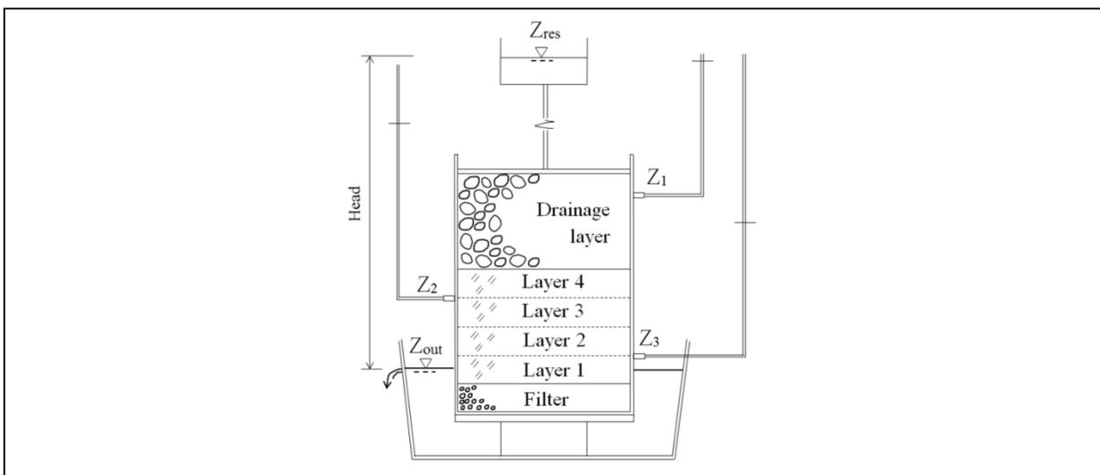
**Figure 1:** Schematic of the test apparatus (not to scale).
