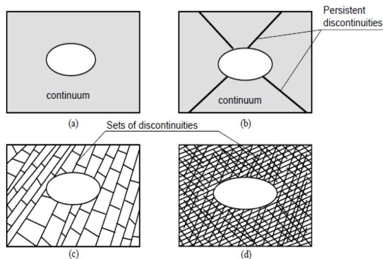
**Figure 1:** Selection of different numerical methods: (a) continuum method; (b) continuum with fracture element or discrete method; (c) discrete model; and (d) continuum method with equivalent properties [2].
