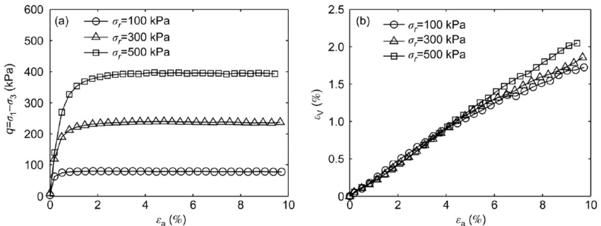
**Figure 4:** DEM simulation of the triaxial extension of Chende sand under different confining pressures: (a) Stress-strain behavior; (b) volumetric strain-axial strain response [29].
