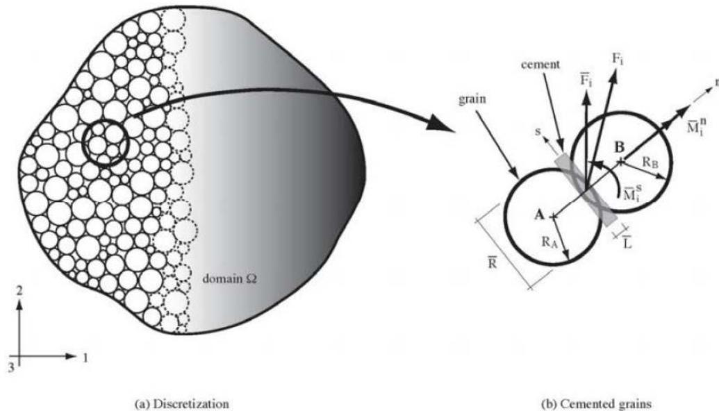
**Figure 2:** Particulate DEM model [14].
