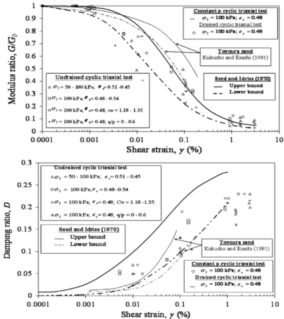
**Figure 5:** Comparison of shear modulus and damping ratio obtained from numerical tests with standard curves [30].
