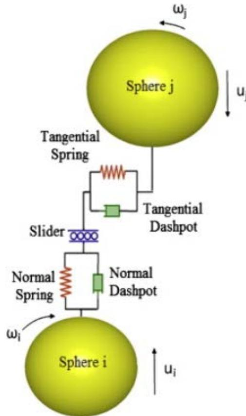
**Figure 3:** Schematic of the constitutive law of normal and shear contact forces between two particles [7].
