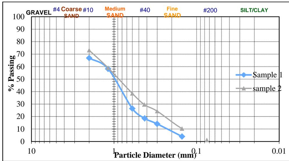
**Figure 1:** Grain Size Distribution Curve of Sample 1 and Sample 2
